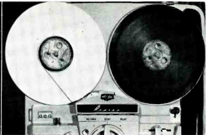
Here, in direct comparison with the "regular" system, is the setup expanded so a full hour can be recorded at 7½ ips. I'll readily admit it looks a bit crowded, but this seems a small penalty to pay for having a complete hour of recording to a "side."
